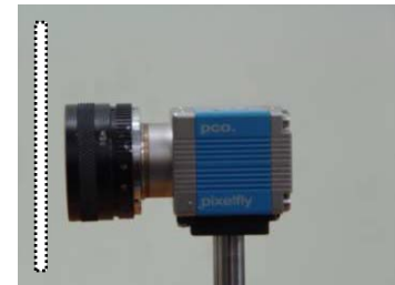
DRZ-phosphor and CCD camera
