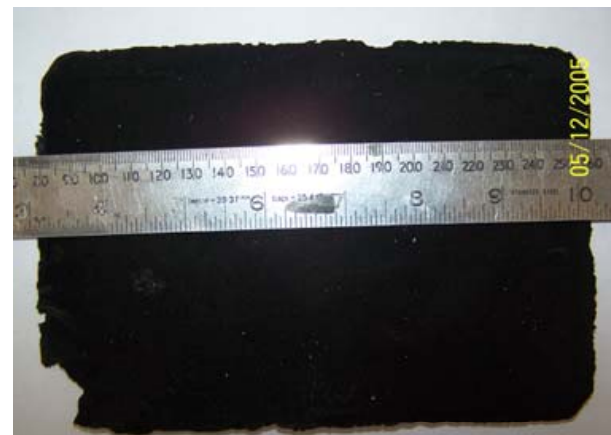
Carbon Foam Electrode ( 125 x 80 mm)
