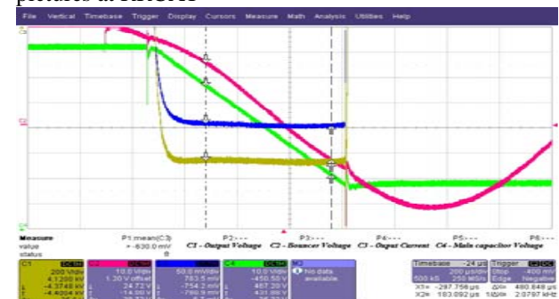
Figure 5 – Obtained output during initial run, at resistive load, representing klystron impedance. Waveforms represent C1:Output voltage C2: Bouncer voltage C3: Output Load current C4: Main Capacitor voltage
