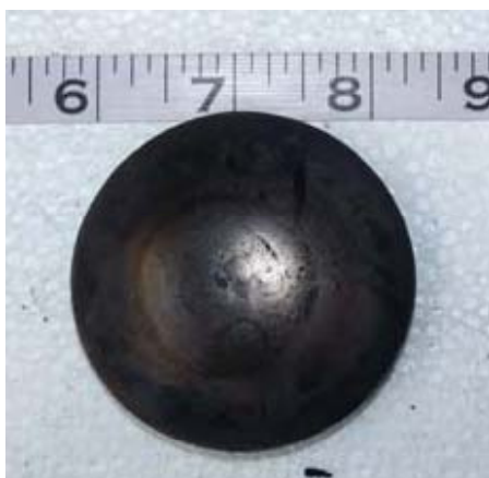
Pt-Loaded Carbon –silica composite cylinders and disc
