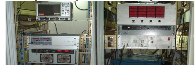
Figure 3. Photo on left: Charging/Filament Supplies photo on right: trigger, controls and interlock system of modulator at RRCAT.
