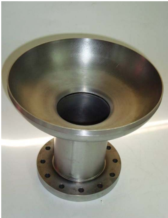
Welding of Beam pipe to Half Cell
