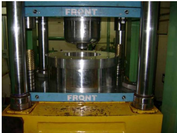
Loading arrangement of dies on the 200 Ton Hydraulic Press at RRCAT
