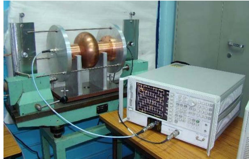
Bead Pull Measurement Setup for Assembled Cavity
