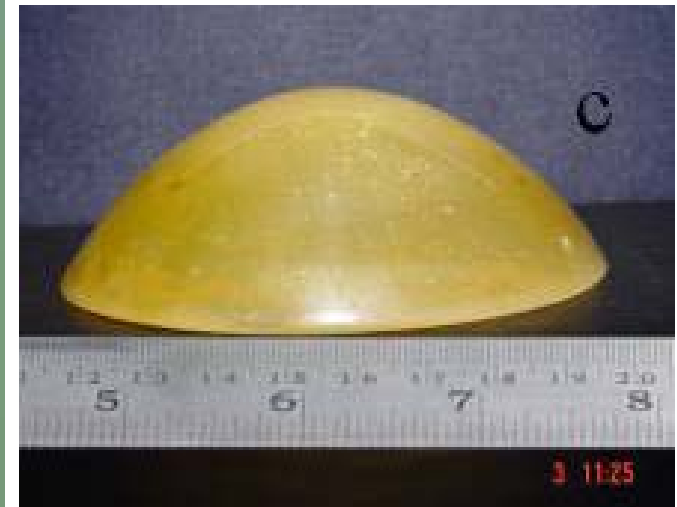
(a) SLN Single Crystal, (b) Oriented KDP crystal & (c) free-standing ZnS dome
