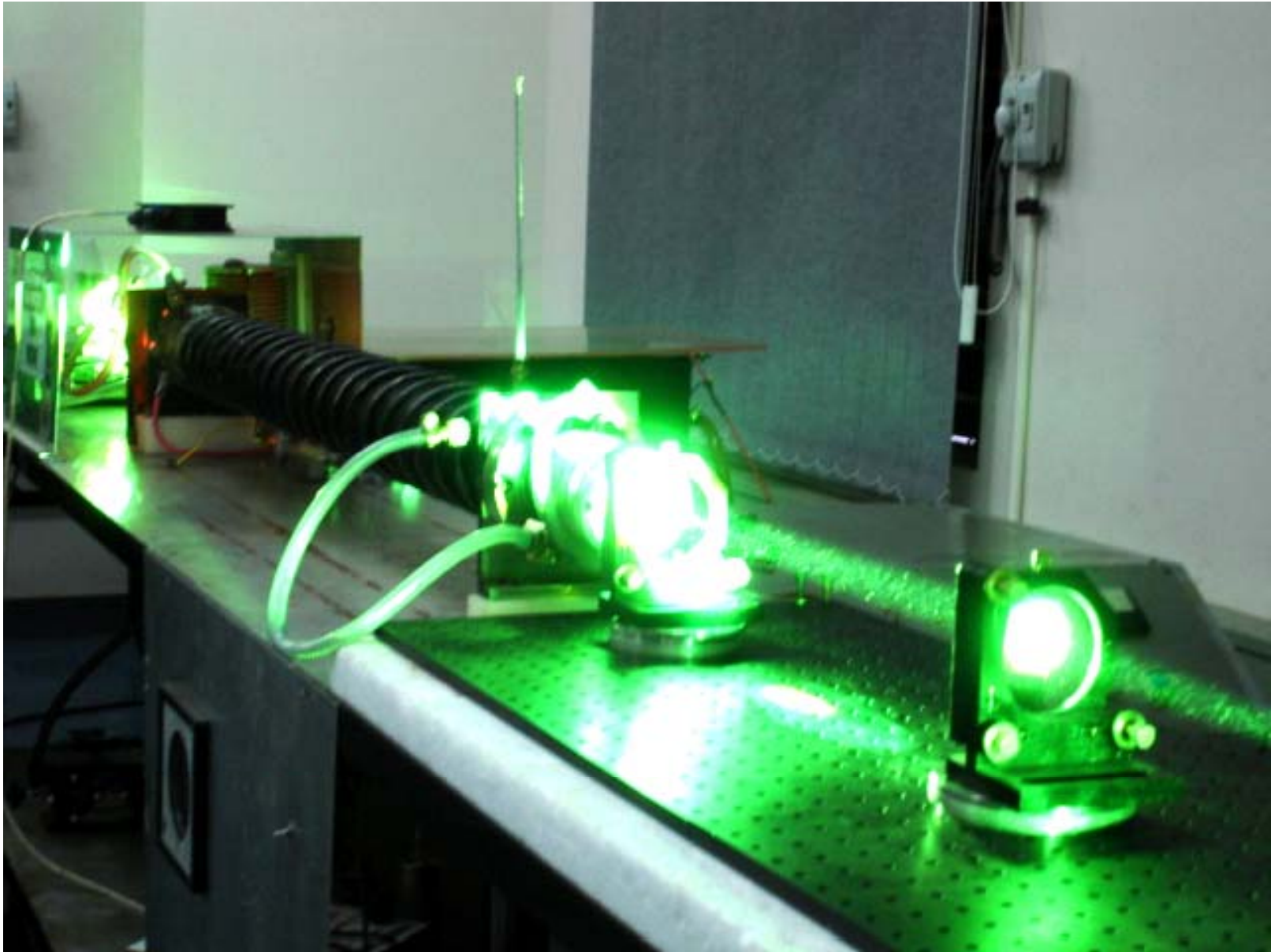
A 60 W prototype version CuHyBrID laser
