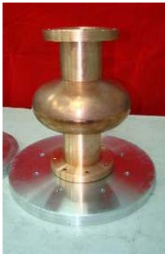
Assembled Cavity with beam pipe & Flanges
