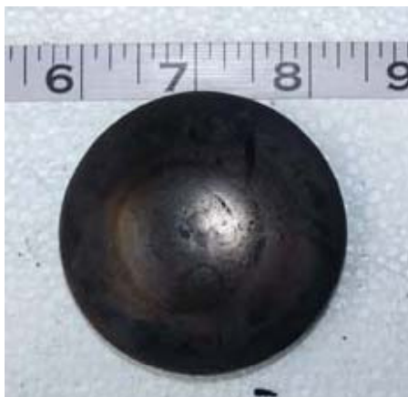
Pt-Loaded Carbon –silica composite cylinders and disc
