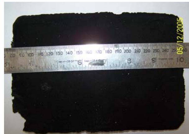
Carbon Foam Electrode ( 125 x 80 mm)
