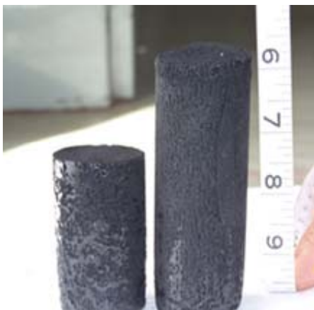
Pt-Loaded Carbon –silica composite cylinders and disc
