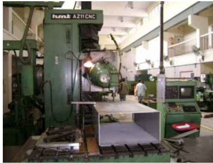
Preparation of WR 2300 full height W/G structure
