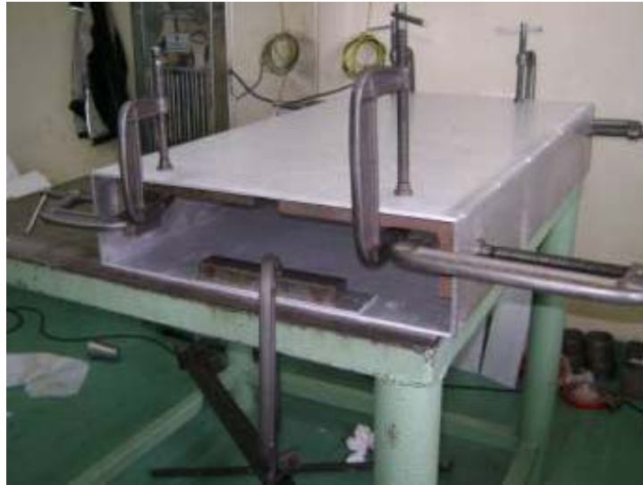
Preparation and welding of WR 2300 half height W/G structure
