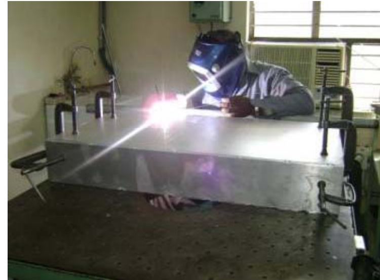
Preparation and welding of WR 2300 half height W/G structure
