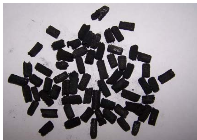
Raschig Ring Morphs of Pt-Carbon Composite Catalyst.
