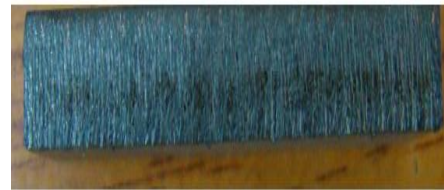
Laser cut surface in air Heat affected zone : 370 \mu m
