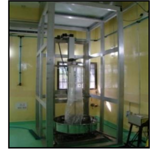
High pressure rinsing Set up
