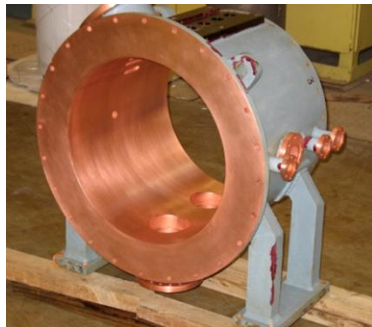
Copper plating of DTL Tank of LEHIPA
