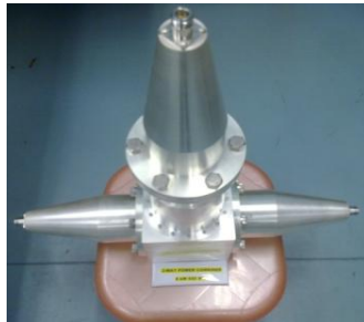
2-way 20 kW Power Combiner
