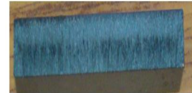
Laser cut surface underwater Heat affected zone : 210 \mu m
