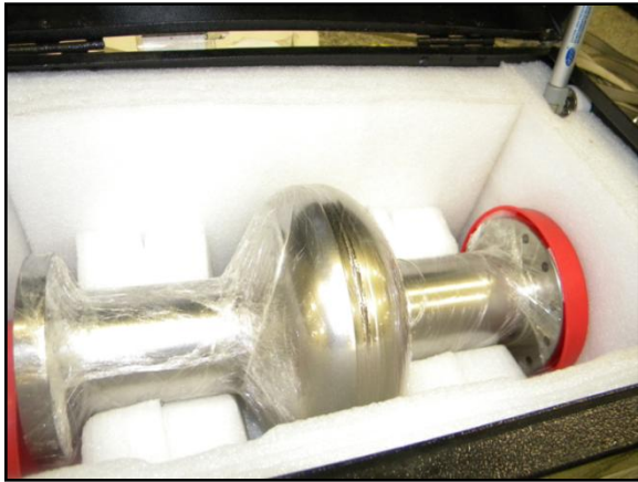
1.3 GHz Nb Single Cell Niobium Cavity developed in India (RRCAT / IUAC)
