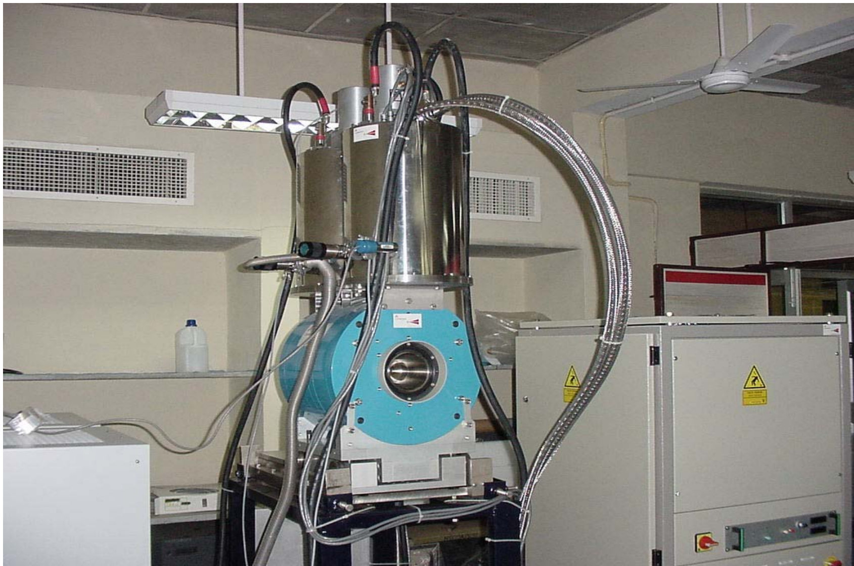
Closer view of the HTS-ECR source with cryotips on top
