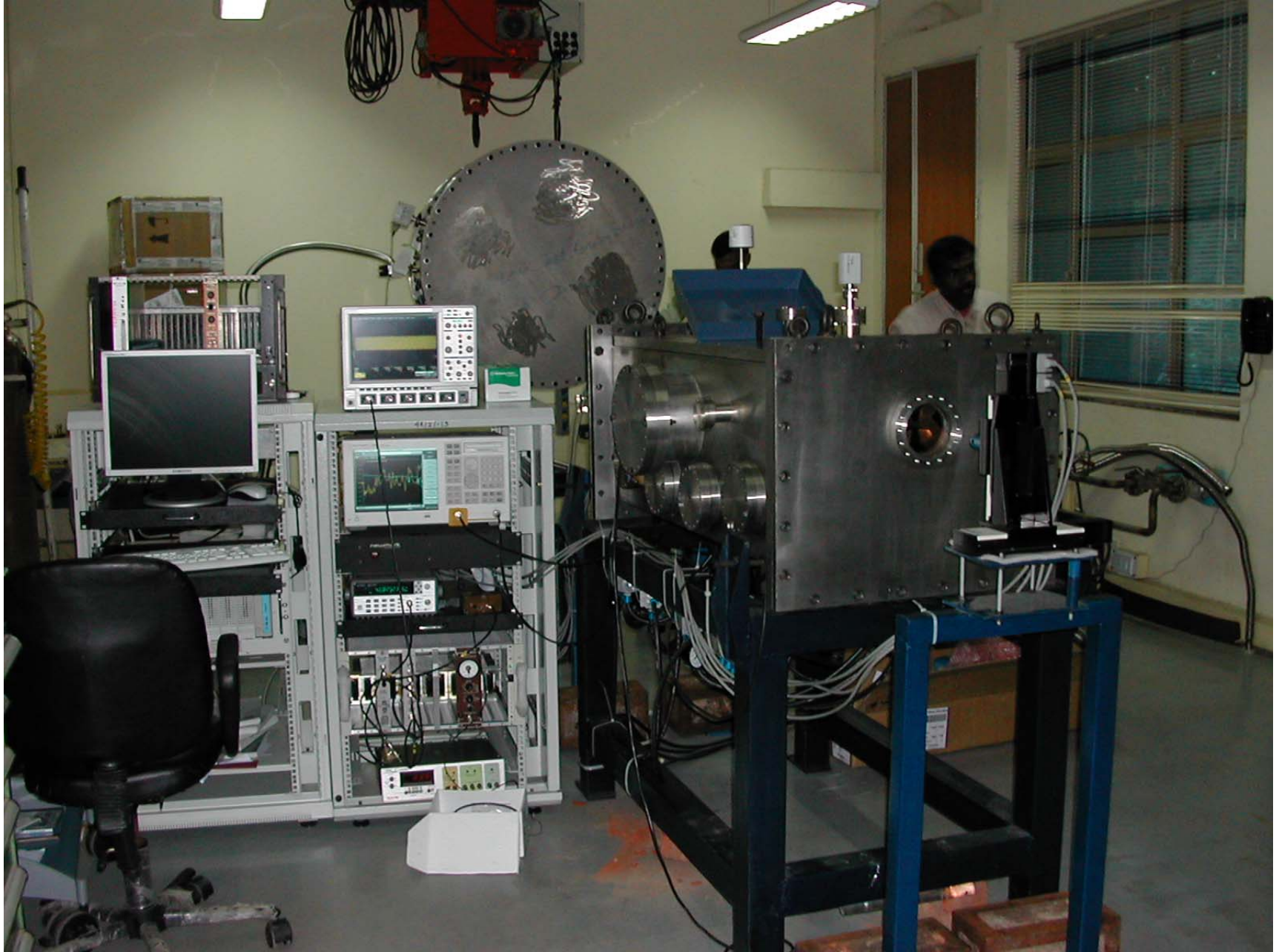
Testing of modulated vanes of RFQ
