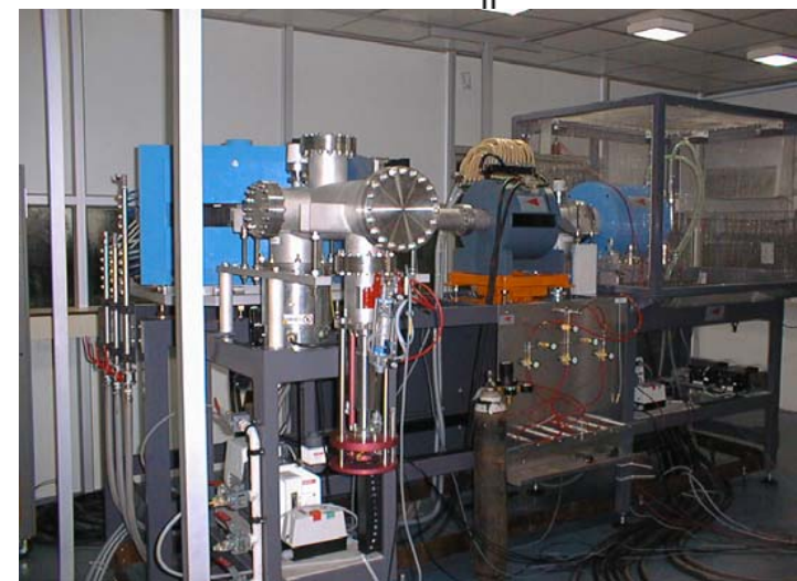
LAYOUT OF HORIZONTAL SECTION OF INJECTION LINE FOR VEC K-500 SUPERCONDUCTING CYCLOTRON
