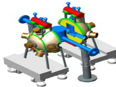
4\pi neutron multiplicity detector
