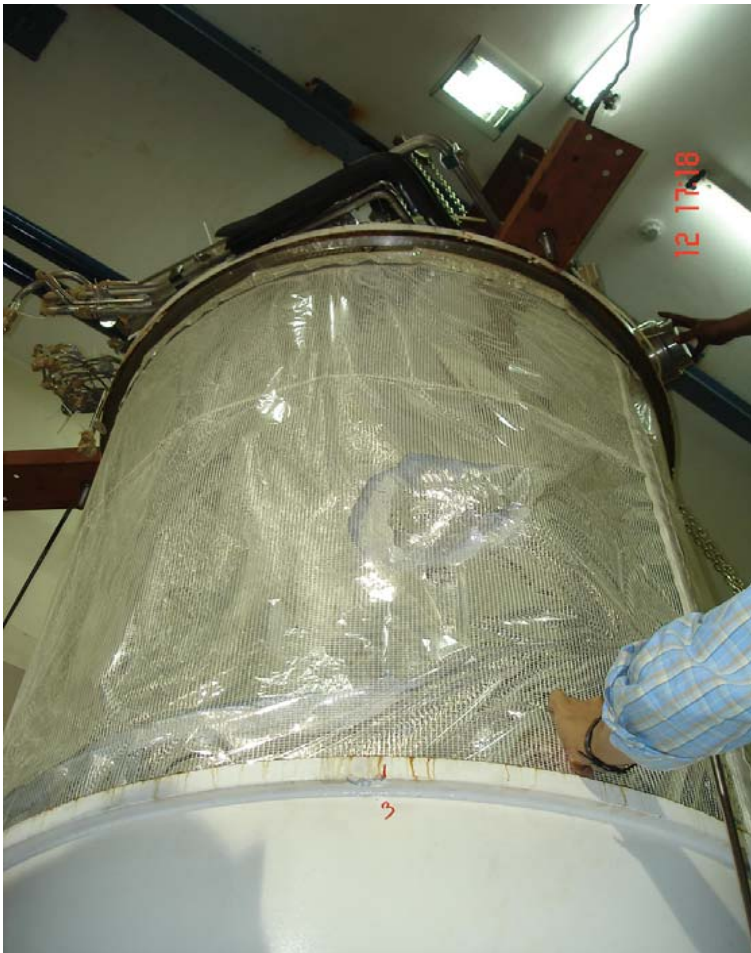
Cold Box With Exterior MLI
