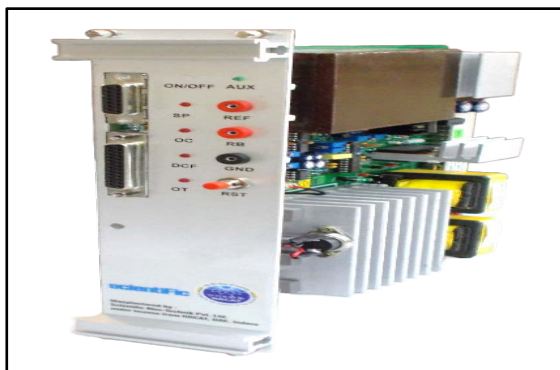
Power converter card.
