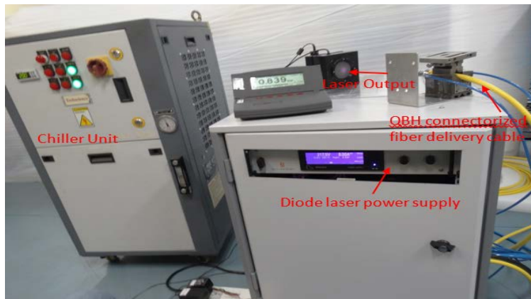
1 kW all-fiber Yb-doped CW fiber laser at 1080 nm.
