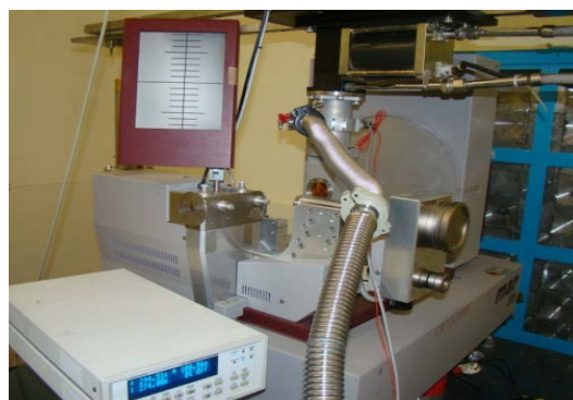
Fig. 7: The closed cycle cryostat based sample cooling stage installed at the image plate of the angle dispersive x-ray diffraction (ADXRD) beamline (BL-12).
