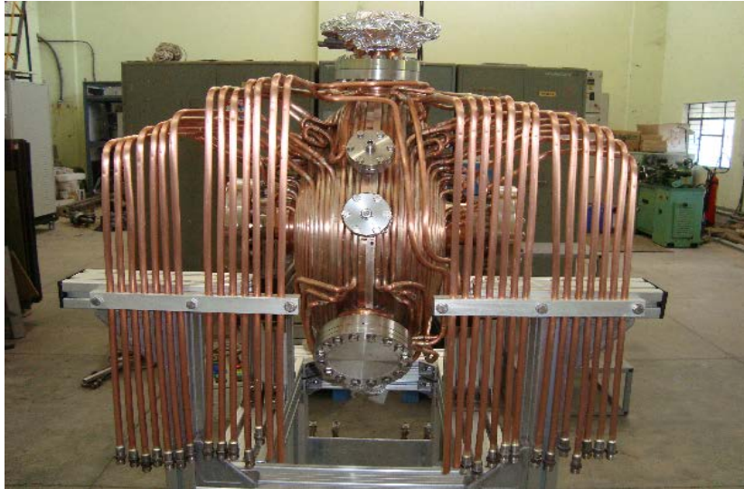
Fig. 20: High purity copper radio-frequency cavity at 505.8 MHz with copper cooling coils.
