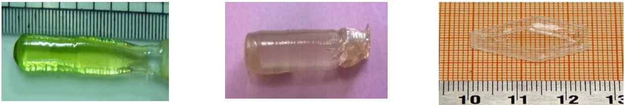
Fig. 59: Photographs of some high optical quality crystals grown using different techniques. (a) Cr co-doped \text{YVO}_4 , (b) \text{Sr}_{0.61}\text{Ba}_{0.39}\text{Nb}_2\text{O}_6 (SBN), (c) trans-stilbene.
