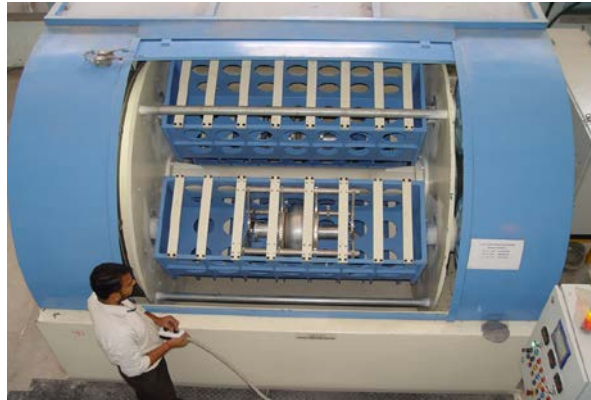
Fig. 16: Centrifugal barrel polishing machine loaded with single-cell 650 MHz cavity.
