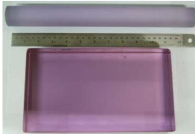
Fig. 37: A typical Nd:glass slab and a 40 mm diameter, 310 mm long Nd:glass rod made from a similar slab.
