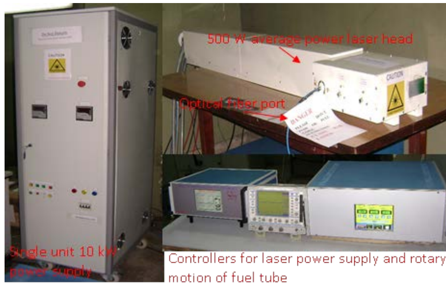
Fig. 31: 10 kW peak power fiber coupled pulsed Nd:YAG laser for IGCAR.
