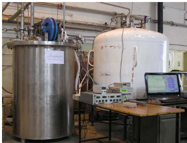
Fig 18: Indigenously developed helium liquefier of 35 litre/hr capacity.
