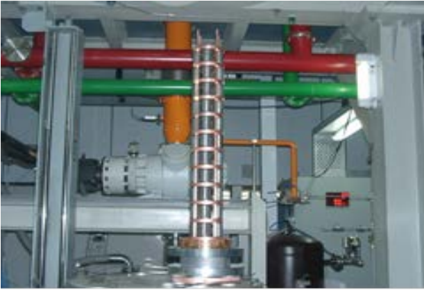
Fig. 25: The plane wave transformer linac for the infra-red free electron laser.
