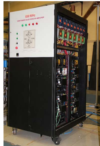
Fig. 64: The 30 kW, 650 MHz solid state amplifier developed under the Indian Institutions- Fermilab Collaboration.
