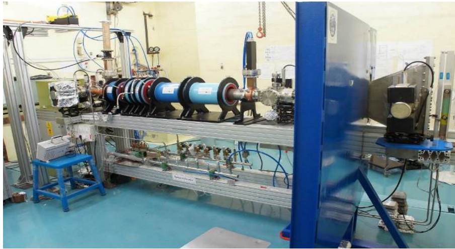
Fig. 24: The 10 MeV industrial linac. The linear accelerating structure, focusing magnetic elements and the beam scanner can be seen.
