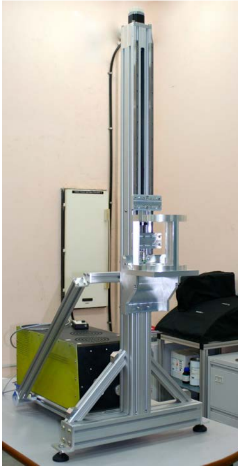
Fig. 57: The laser based fiber drawing system
