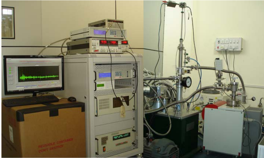
Fig. 62: Experimental facility of Resonant Ultrasound Spectroscopy for the measurement of the elastic constants materials at low temperatures (2-300 K) and in high magnetic fields (up to 70 kOe).
