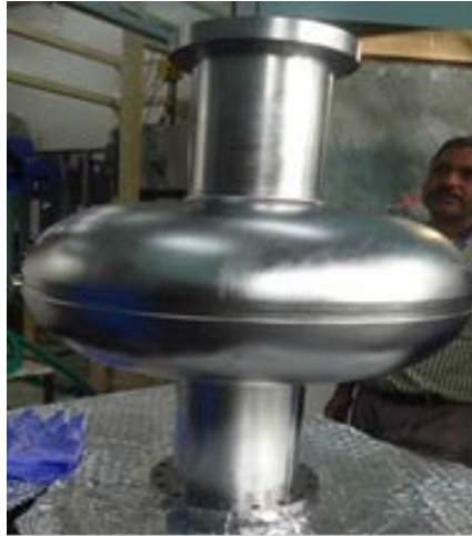
Fig. 17: The 650 MHz laser-welded superconducting radio-frequency cavity.
