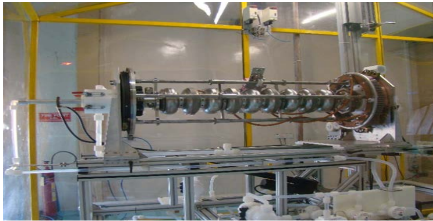
Fig. 14: Electro-polishing of the nine-cell 1.3 GHz superconducting radio-frequency cavity.
