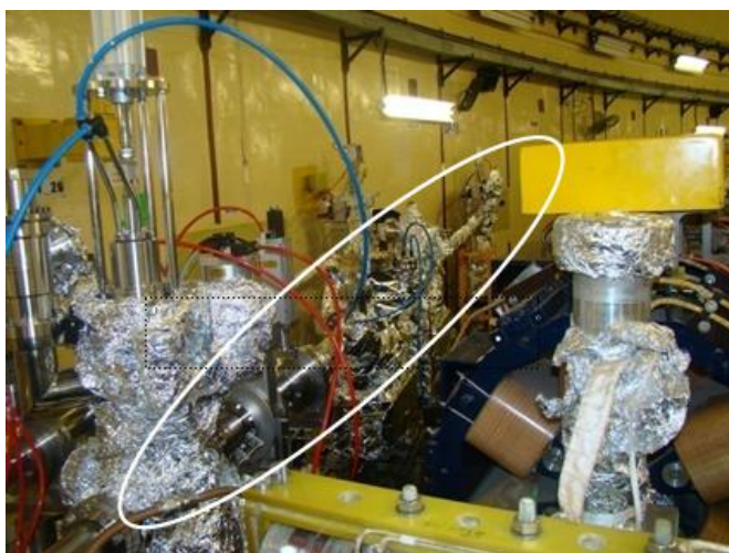
Fig 12: View of the photo emission electron microscope (PEEM) beamline (BL-22) front end that has been installed on the Indus-2 ring.
