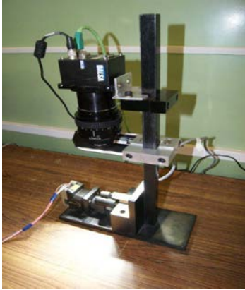
Fig. 52 : The line camera system for fuel pellet inspection.
