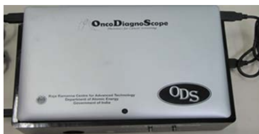
Fig. IV.9.1: Tablet computer based, user-friendly cancer diagnostic system.
