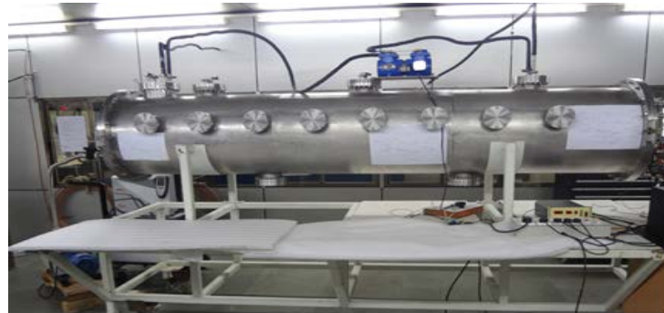
Fig. II.6: Table top version of the liquid nitrogen powered cold capsule for the reefer application.
