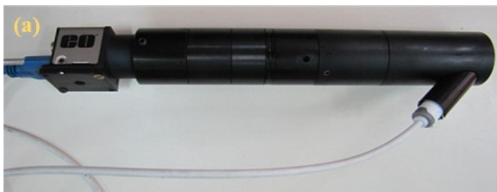
Fig. IV.11(a): Hand held orthogonal polarization spectral imaging setup for in-vivo imaging of micro-vasculature.
