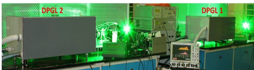
Fig. III.5: Two engineered diode pumped green lasers (DPGL1 and DPGL2) under operation.
