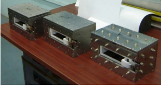
Fig.I.B.8.1.1: Upgraded pulsed injection kicker magnets.
