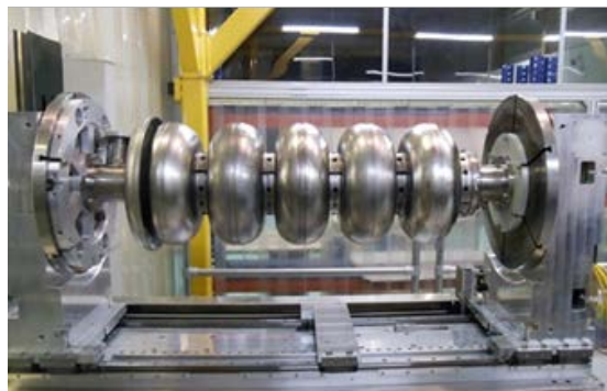
Fig.II.1: First 650 MHz ( \beta=0.92 ) five-cell SCRF cavity developed at RRCAT.
