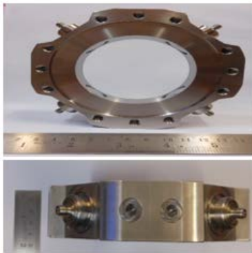
Fig.I.B.8.3.3 : In-house developed ultra-high vacuum compatible FIBPM-152OD (left) and FIBPM-70OD (right).
