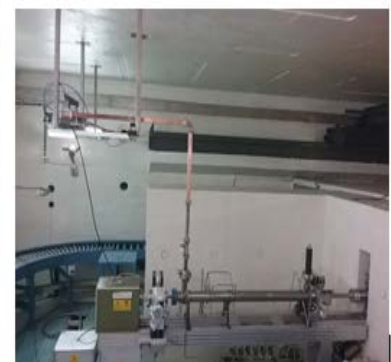
Fig. II.12.2: 6.0 MW microwave system and electron gun installed at ARPF site.
