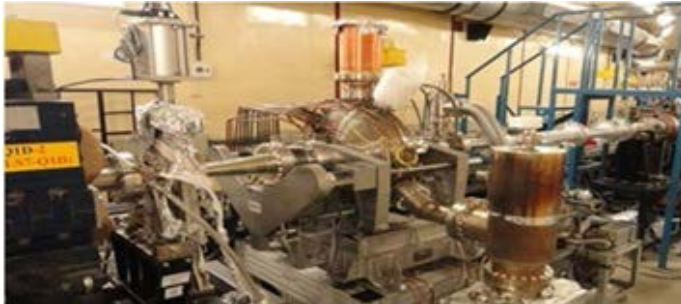
Fig. I.B.1: RF cavity installation in the Indus-2 ring straight chamber.
