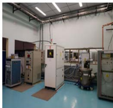
Fig. II.12.2: 6.0 MW microwave system and electron gun installed at ARPF site.
