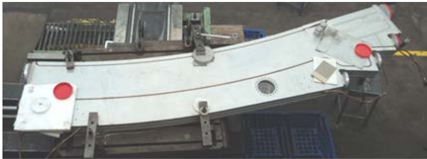
Fig.I.B.8.2: Indus-2 dipole magnet vacuum chamber after modifications.
