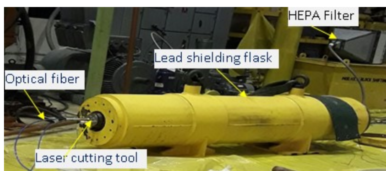
Fig. IV.3: Laser cutting of 18 mm thick end fitting in lead shielding flask.
