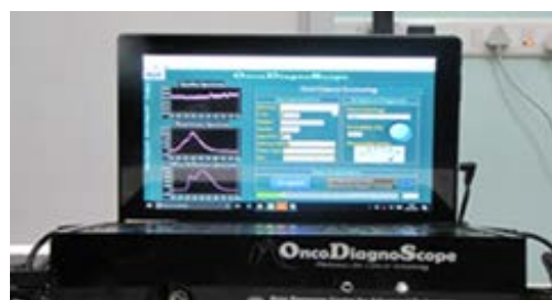
Fig. IV.9.2: A touch screen enabled GUI software for hardware control of the system, data acquisition and data analysis
