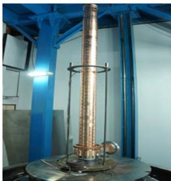
Fig. II.12.1: Vacuum brazing of complete 10 MeV structure.
