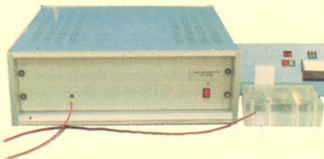
N 2 laser with fiber optic beam delivery system.
