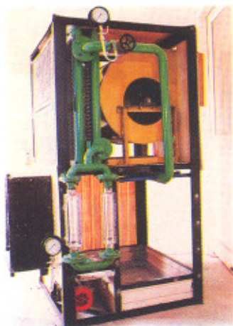
Energy Recovery Unit Developed at CAT
