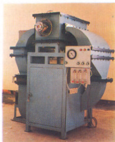
High rep rate TEA CO 2 laser developed at CAT
