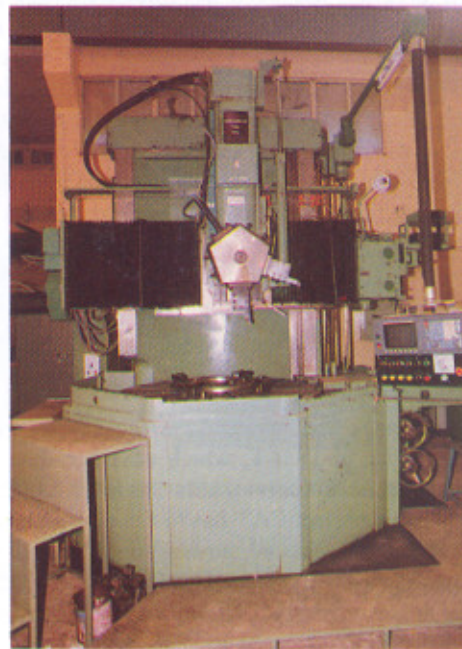
CNC Vertical Turret Lathe installed at CAT
