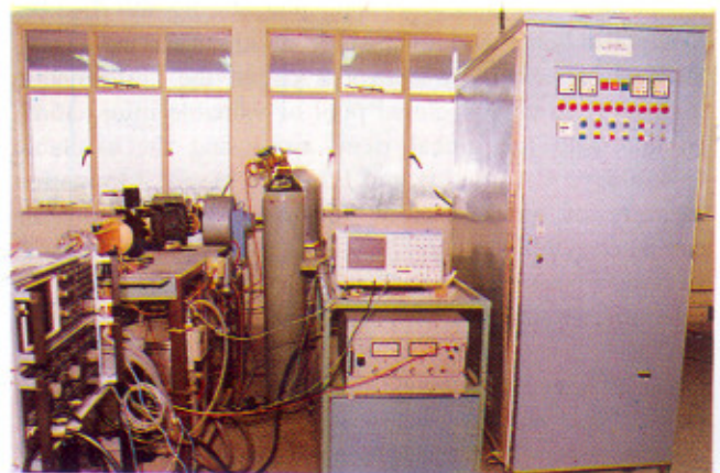
2MW Indigenous magnetron under going life test at microwave test facility at CAT.
