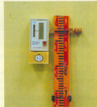
Fig. L.2.1 Scanner and Scale unit
