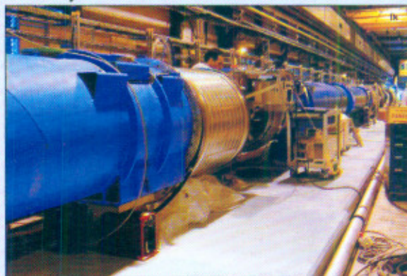
Fig. A.7.1 The prototype jacks under a cryo-dipole at LHC test string-1 at CERN
