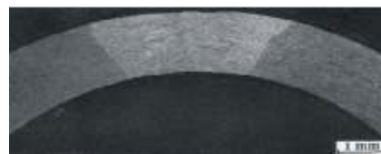
Fig.L.12.1 Fusion zone microstructure of LCW specimen. Inset: Low magnified view of laser weldment.
