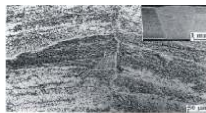
Fig.L.12.2 Cross-section of bend tested LCW specimen
