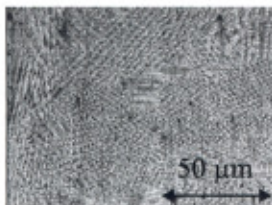
Fig. L.14.2 Microstructure of LRM fabricated Inconel-625 specimen
