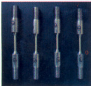
Fig. L.14.1 LRM fabricated machined tensile specimen
