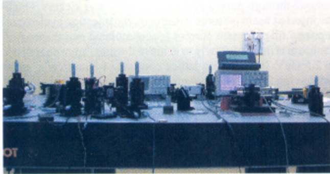
Fig. L.17.1 Experimental setup of DEPSS laser operating with 535mW of SLM output power at 1064nm
