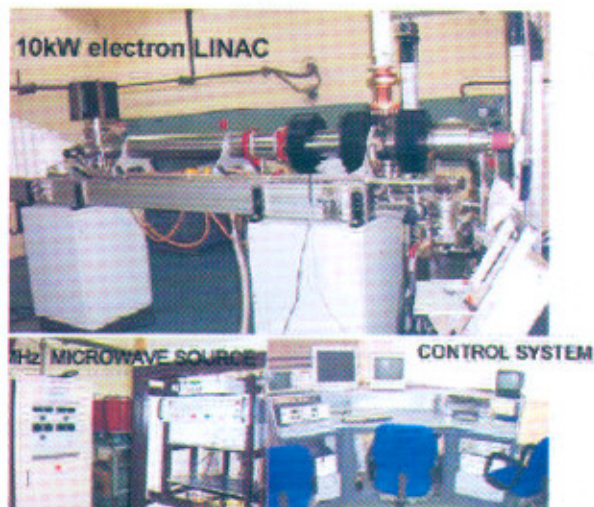
10 MeV, 10 kW LINAC for radiation processing application
