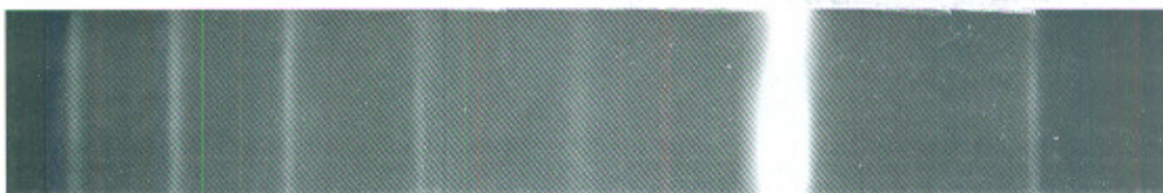
Coherent soft X-ray radiation generated as high order harmonics using Ti-sapphire laser. The harmonic at 61 nm shows 200X intensity enhancement
