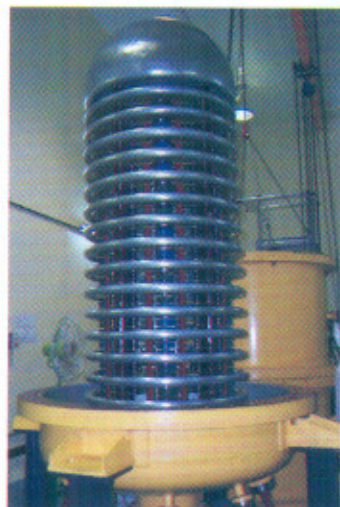
750 keV, 20 kW DC accelerator for surface irradiation of agriculture products and radiation processing application
