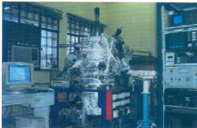
Ultra high vacuum electron beam evaporation system for fabricating x-ray mirrors
