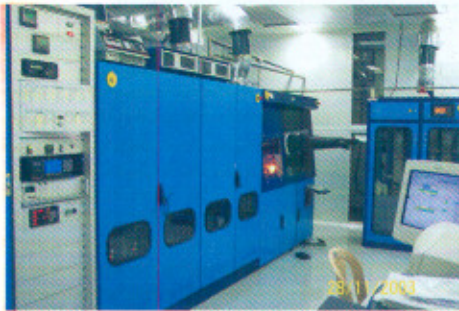
MOVPE set up being used for making semiconductor laser diode
