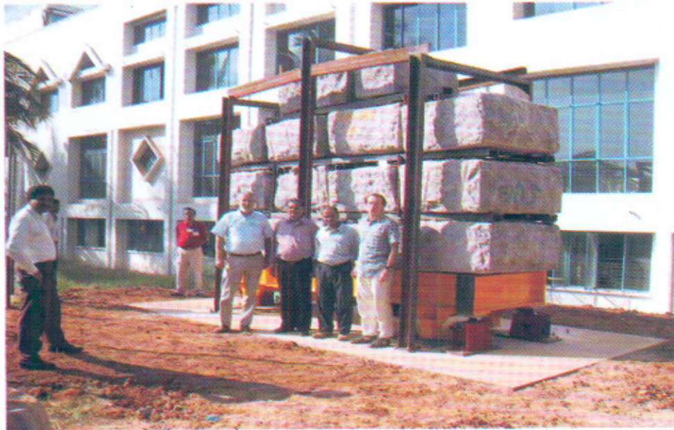
Precision alignment jacks being tested at AAL, Bangalore before shipment to CERN
