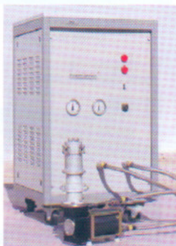
Closed cycle cryocooler capable of producing a temperature of 10K-30K
