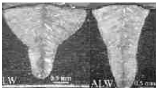
Fig. L.12.3 Comparison of key-hole welds produced by LW and ALW.
