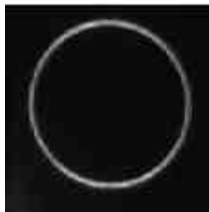
Fig. L.6.1 CCD image of the hollow beam generated by axicon mirror.
