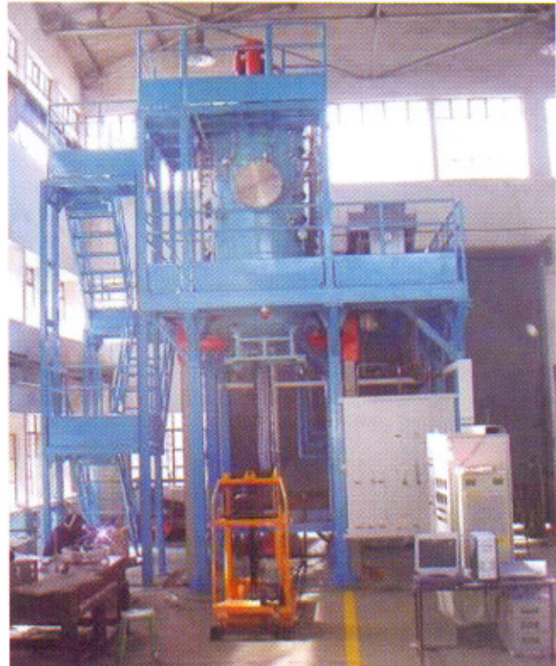
Fig.I.3.1: Photograph of the vacuum brazing furnace.
