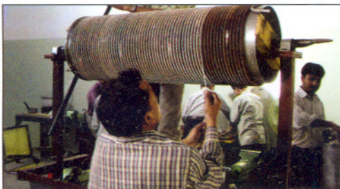
Fig. A. 3.1: Winding of finned-tubes over the inner shell of heat exchanger for 300 - 80 K temperature range.
