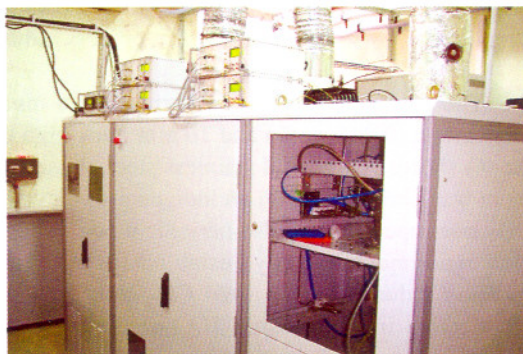
Fig. L.6.2: A view of MOVPE system with the AIO control units in operation
