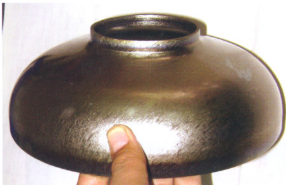
Fig. A.8.1: Niobium half cell formed at RRCAT
