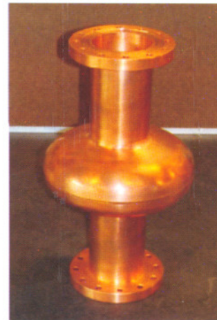
Fig. A.8.3: Single cell copper cavity formed at TRIUMF using the tooling developed at RRCAT.
