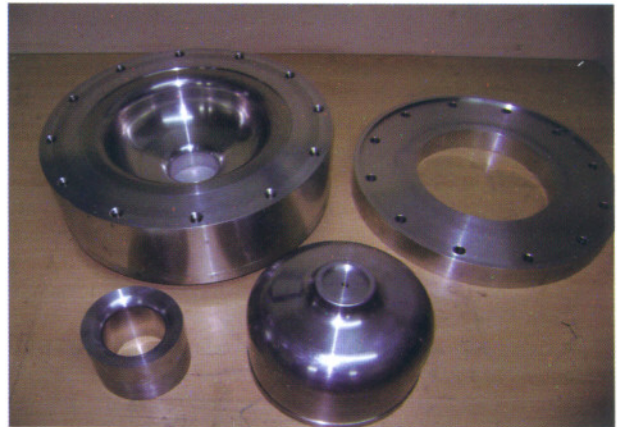
Fig. A.8.2: Forming tooling for centre cell of the Cavity
