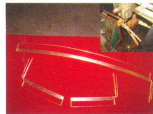
Fig. A.6.2: Machined septum magnet coil. Inset shows machining of end connections on EDM wire cut
