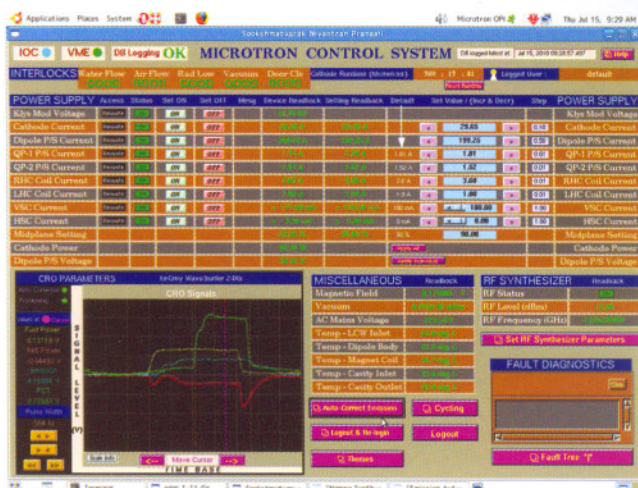
Fig. A.7.1: The Microtron Control GUI developed in EPICS
