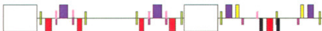
Fig.A.1.1: One unit cell of Indus-2 : empty rectangles - dipoles; blue-focussing quadrupoles; red- defocussing quadrupoles; yellow-focussing sextupoles; black-defocussing sextupoles; green- BPIs ; magenta- horizontal steering magnets and pink-vertical steering magnets.
