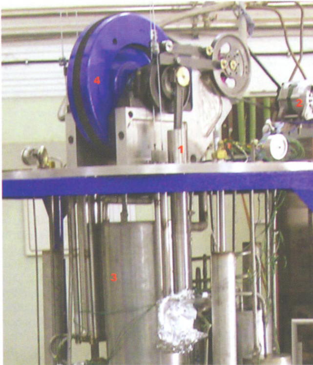
Fig.T.1.2: Photograph showing expansion engine along with heat exchangers and auxiliary components. 1. Cryogenic Expander, 2. Work extraction mechanism, 3. 1 st heat exchanger, 4. Flywheel
