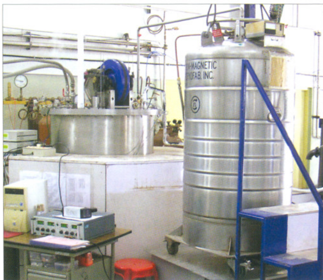
Fig.T.1.7: Photograph shows Helium Liquefier developed at RRCAT
