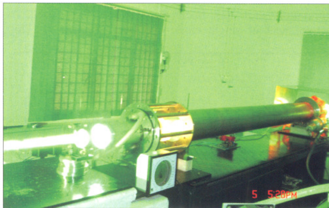
Fig. T.2.8: A 110 W, 18 kHz repetition rate Copper HyBRID laser developed at LSED, RRCAT
