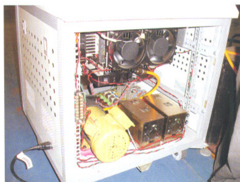
Fig.T.2.7 : The temperature controlled dye circulation system along-with TEC, (a) Block diagram, (b) Assembled system
