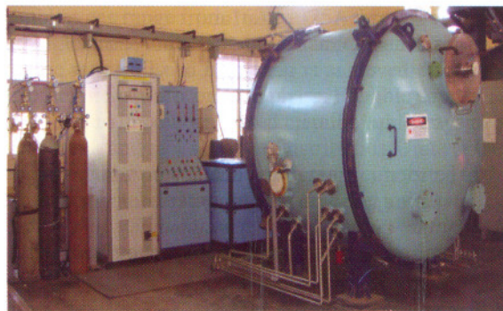
Fig.L.7.1: Renovated 5kW CW CO 2 laser
