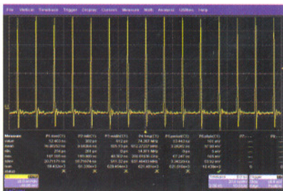
Fig.L.9.4. Temporal spectra of KLM laser recorded with 0.5 ns photodiode FPD510.
