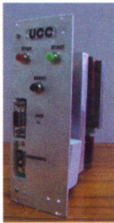
Fig. T.3.22: Photograph of ultracapacitor charger and charging voltage (top) and current (bottom) waveforms.
