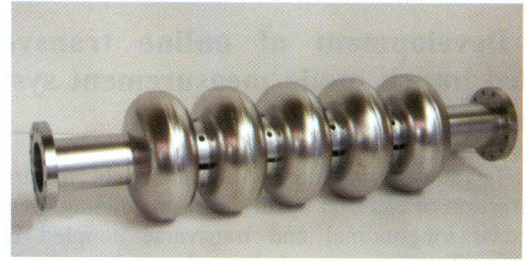
Fig. A.3.3: 1.3 GHz Five cell SCRF cavity
