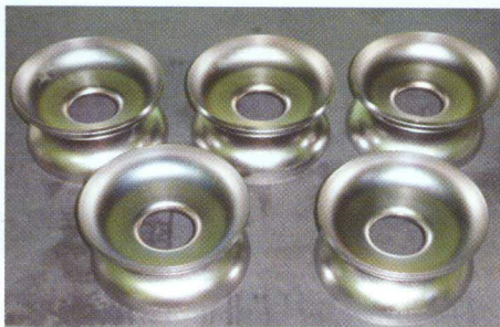
Fig. A.3.1: Dumbbells for 1.3 GHz Five SCRF cavity
