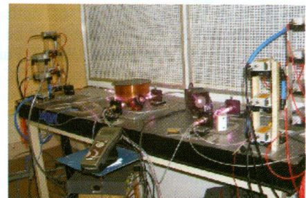
Fig. L.3.2: A table-top view of 160 W single transverse mode CW fiber laser.
