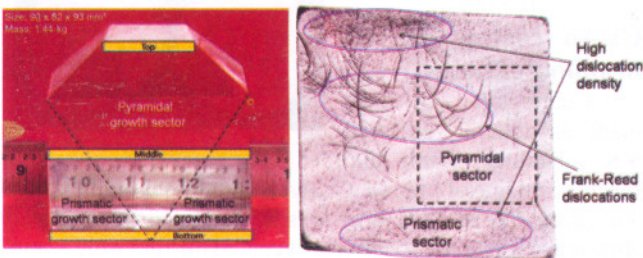
Fig L.9.2. Large size KDP crystal and X-ray topograph of (316) planes for plate from middle of the crystal.
