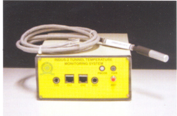
Fig.A.5.2: TTMS controller along with temperature sensor probe
