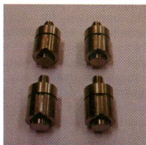
Fig.A.2.3: Laser welded electrode sub-assemblies
