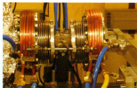
Fig. A.2.5: IDBPI installed with undulator in Indus-2
