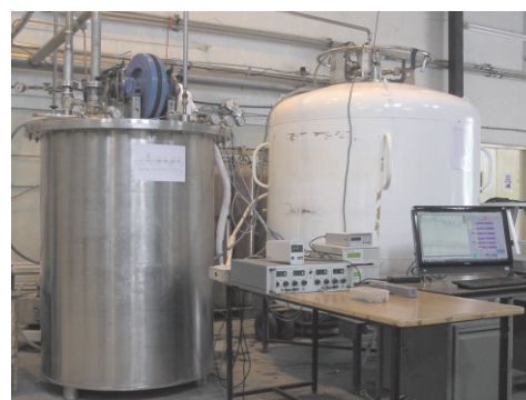
Fig. A.4.3: Photograph showing indigenous helium liquefier liquefying helium in a 1,000 litre Dewar
