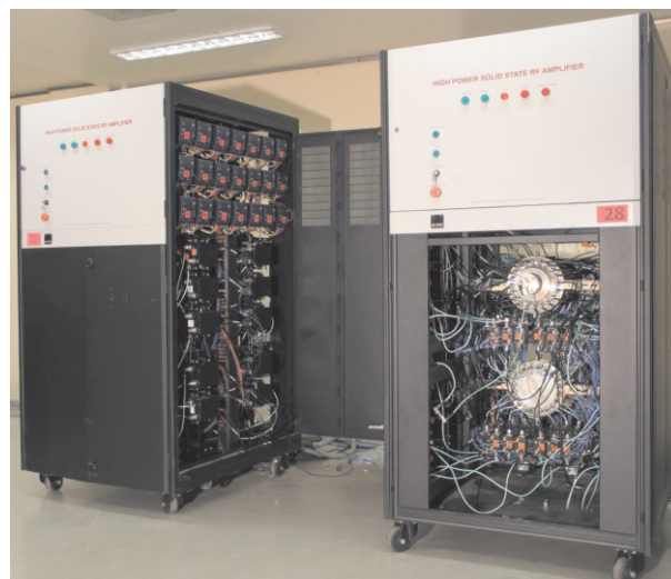
Fig.A.9.2: Fabricated 650 MHz, 30 kW solid state RF amplifier
