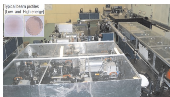
Fig.L.2.1: Compact 50 J Nd:phosphate glass laser system at Laser Plasma Division. Inset also show typical beam profiles at low and high pulse energy regimes.
