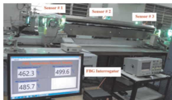
Fig. L.4.2:FBGs based distributed temperature sensors for monitoring temperature of CuBr laser tube
