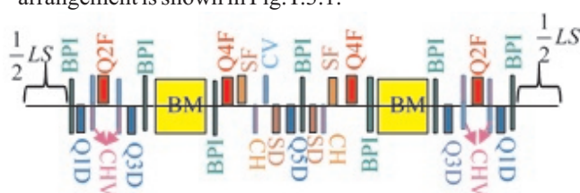
Fig. T.3.1: Unit cell of Indus-2, BM: Dipole magnet; Q1D, Q3D, Q5D: Defocusing quadrupole magnets; Q2F, Q4F: Focusing quadrupole magnets; SF: Focusing sextupole magnets, SD: Defocusing sextupole magnets; CH: Horizontal steering magnets, CV: Vertical steering magnets, CHV: Combined horizontal and vertical steering magnets; BPI: Beam position indicator, LS: Long straight section
