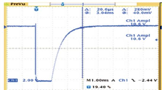
Fig. A.1.2: Bolometer trace showing saturated IR signal
