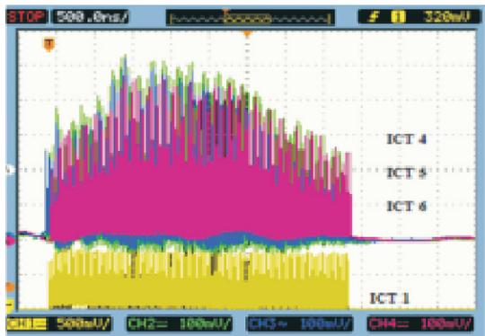
Fig. A.1.1: ICT signals at different locations along the electron beam transport line
