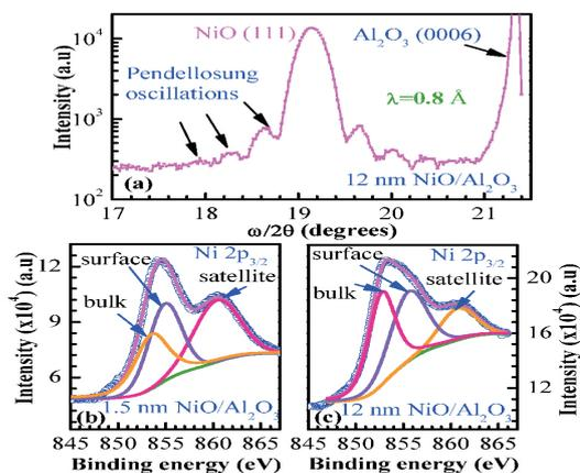
Fig. A.8.1: (a) ω/2θ scans from ~12 nm thick NiO layer deposited on Al<sub>2</sub>O<sub>3</sub> substrate. The Ni 2p<sub>3/2</sub> core level spectrum for (b) ~1.5 nm (c) ~12 nm thick NiO layers.
