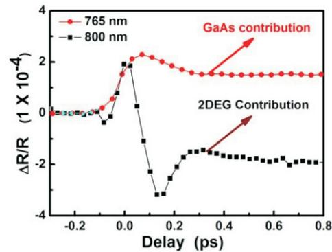
Fig. L.10.3: Room temperature TR curves for the  $Al_{0.7}Ga_{0.3}As$ -GaAs heterostructure showing the individual contributions from the GaAs and 2DEG layers obtained by selecting appropriate wavelengths as per Fig L.10.2.
