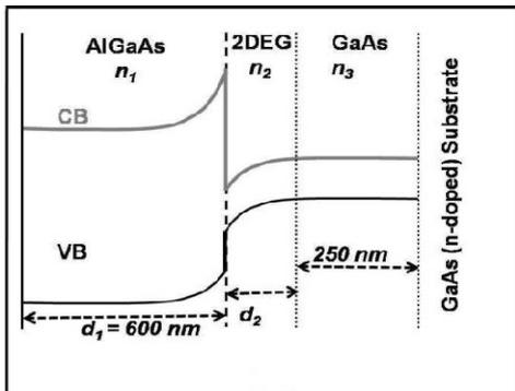
Fig. L.10.1: Band bending diagram.  $n_1$ ,  $n_2$  and  $n_3$  are refractive indices for AlGaAs, 2DEG region and GaAs respectively.  $d_1$  and  $d_2$  are thickness of AlGaAs and 2DEG layer respectively.
