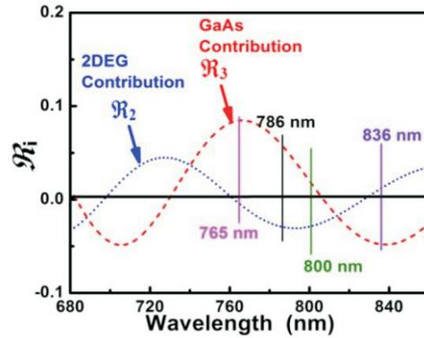
Fig. L.10.2: Calculated wavelength dependence of the contribution to the linear reflectivity from the GaAs and 2DEG layers of the heterostructure.
