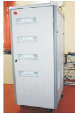
Fig. L.2.3: 20 kW modular SS-RFPS
