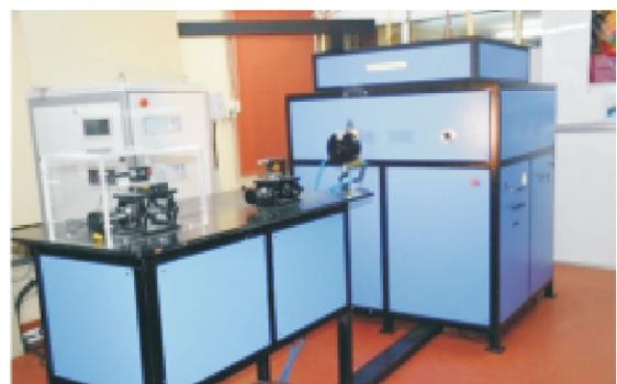
Fig. L.4.4: Upgraded 2 kW RF-FAF CO<sub>2</sub> laser
