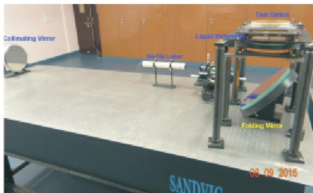
Fig. L.5.2: Photograph of the Liquid reference Fizeau interferometer
