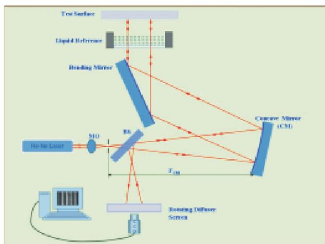
Fig. L.5.1: Schematic of the interferometer system
