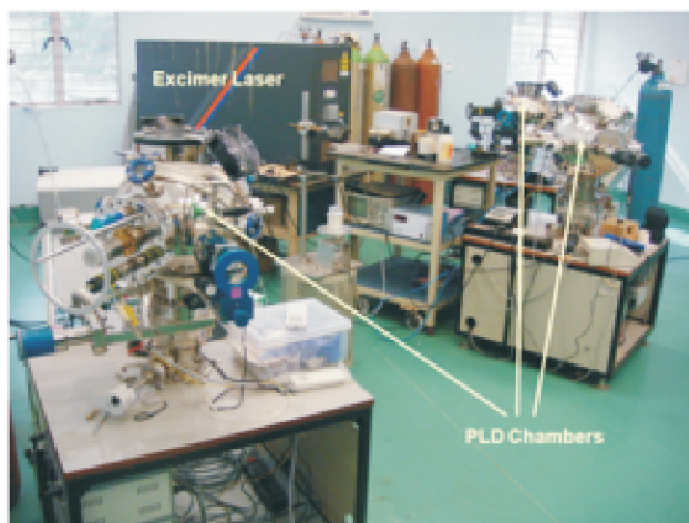
Fig. T.2.2: Image of PLD setup at LMPD, RRCAT consisting of KrF excimer laser and PLD chambers.
