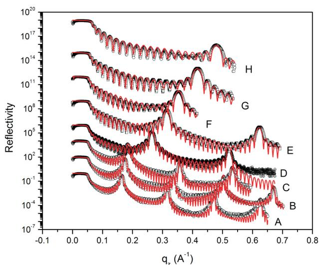
Fig. T.3.4: X-ray reflectivity curves both experimental (open circles) and fitted (solid lines) as a function of wave vector transfer 'q<sub>z</sub> (Å<sup>-1</sup>) for all the as deposited samples (A-H)
