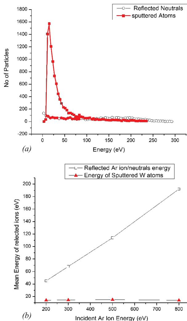
Fig.T.3.1: Top (a) number density and energy distribution of sputtered atoms (red line) and reflected ar ions/neutrals (black line) (b) (bottom). Changes in mean energy of sputtered W atoms (red triangle) and reflected neutrals with the incident Ar ion energy
