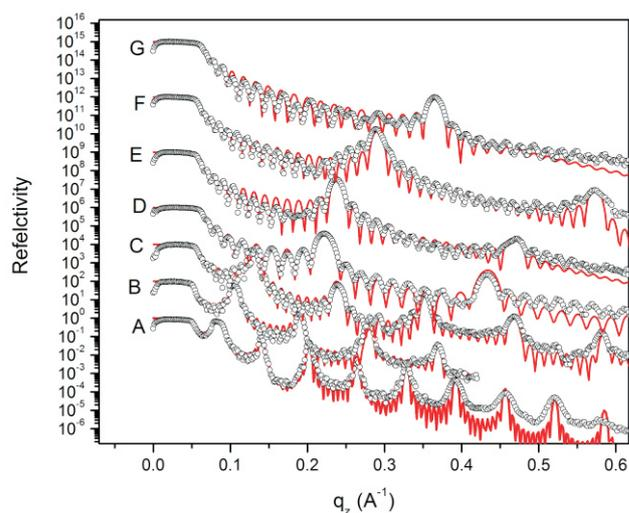
Fig.T.3.2: X-ray reflectivity curves both experimental (open circles) and fitted (solid lines) as a function of wave vector  $q_z$  ( $\text{\AA}^{-1}$ ) for all samples (A-G)
