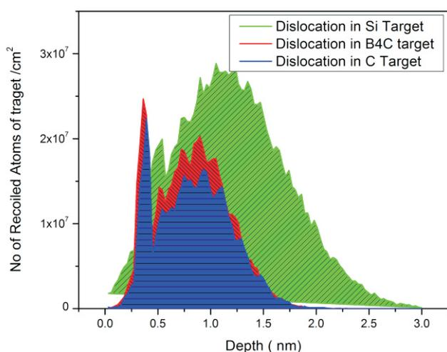
Fig.T.3.3: Damage profile produced due to hitting of 100 eV ions/neutrals on 3 nm layer of Si B<sub>4</sub>C and C layer.
