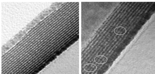
Fig.T.3.6: Cross sectional TEM of sample E ( $D=2.02\text{nm}$ ) and G ( $D=1.52\text{nm}$ )
